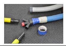
If you do not have a HB300, use tape to temporarily seal the Main W to the end of the extraction line.
