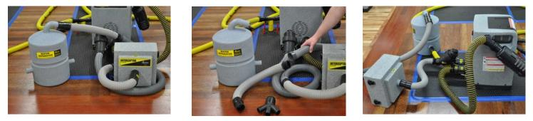
STEP 1: (Left) Install the Interceptor Air In and Out hoses onto the HP unit (as instructed in the Interceptor manual). Remove the Main W from the end of the Air In hose and thread the male end of the Water Separator's hose into the female fitting on the end of the Air In hose.
