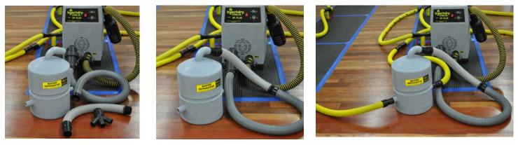
STEP 1: (Left) Remove Main W from the end of your AIR IN main hose (either HP60 or HP-PLUS).
