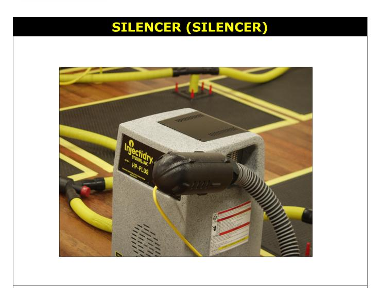
The Silencer is made of ABS plastic and quiets the drying system by about 2 decibels. It actually takes some of the impeller noise out in addition to attenuating the air rush sound. The Silencer attaches to either the Main AIR IN or AIR OUT Hose on the HP60 and the HP-PLUS. *Due to probable high heat output, the Silencer should be elevated from surfaces that could be damaged by heat.*
