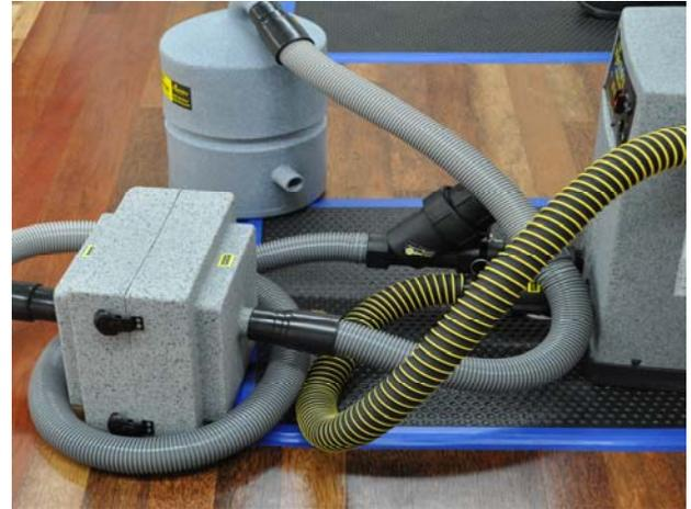
**STEP 1:** If using the Water Separator, before you connect the Interceptor Main Air IN hose to the Interceptor, thread the 2" female fitting (on the end of the Interceptor AIR IN hose) onto the 2" male fitting installed on Water Separator. Push the hose cuff onto the Interceptor.
