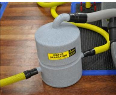
**STEP 2:** Connect up to two of the drying lines to the Water Separators two ports (cap off unused port with end cap plug). We recommend using this method for the first 24 hours after thoroughly extracting with a truck mount (see Water Separator manual).
