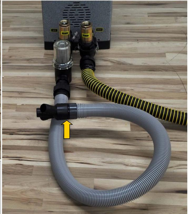
**STEP 2:** Remove and set aside the Main W from the end of the Main Air IN hose from either the HP unit.
