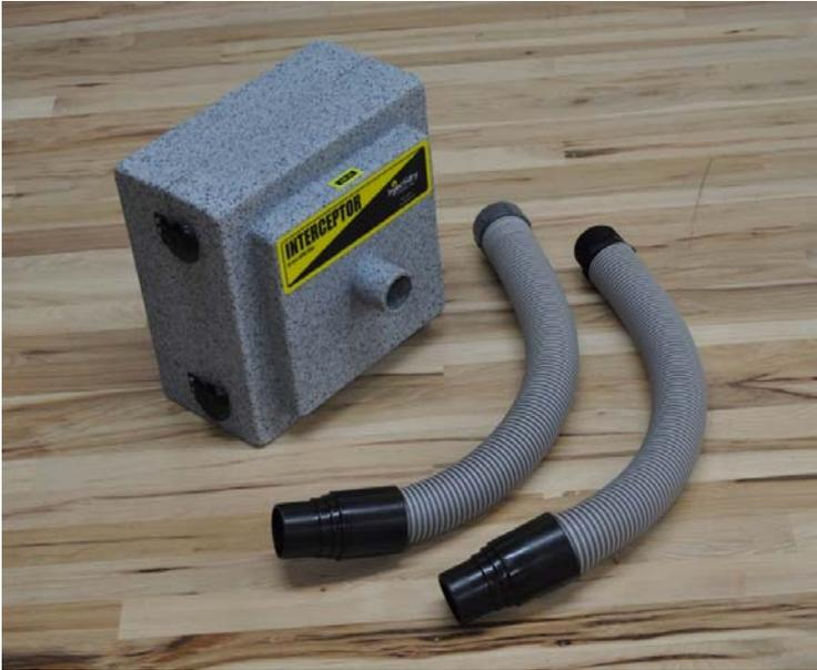
**STEP 1:** Install the Interceptor Air IN Main hose onto the Interceptor HEPA filter. Each hose is labeled with an AIR IN and AIR OUT label. This can get a little confusing, so we recommend following these steps to ensure it is placed in the right order.
