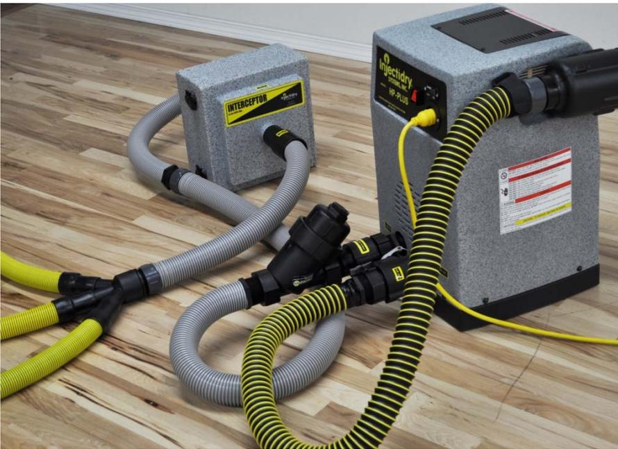
Using the Interceptor HEPA filter will help prevent particulate damage to your machine and prevents cross contamination of mold, pet dander and other allergens.
